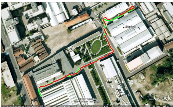
Figure 14: GPS trajectory (red) and SLAM trajectory (green) superposed on the satellite image of the Campus of Bovisa (Milan) where the sequences were acquired
